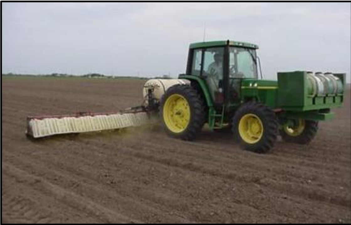
Figure 16. Hooded sprayers reduce spray drift and improve spray efficiency.
