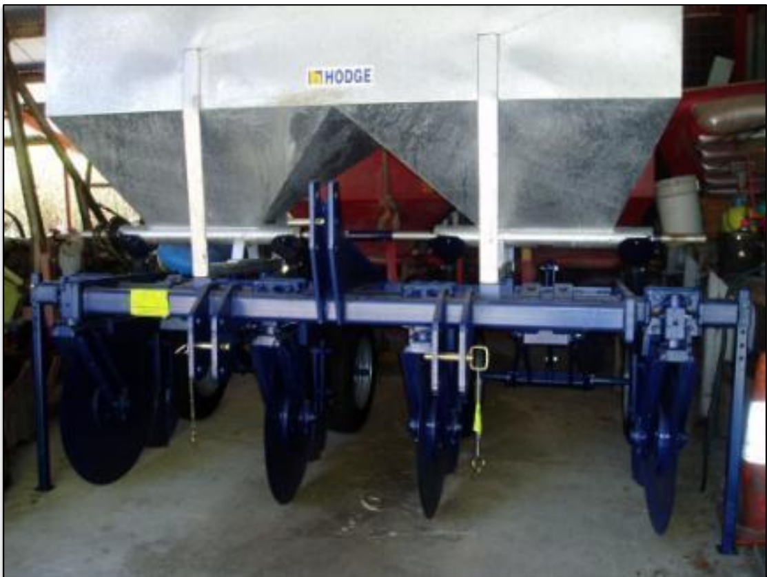
Figure 9. Sub-surface fertilizer applicator places nutrients in the plant root zone.
