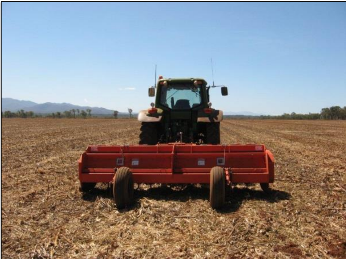
Figure 11. Kronos mulcher returns organic matter back into the soil.
