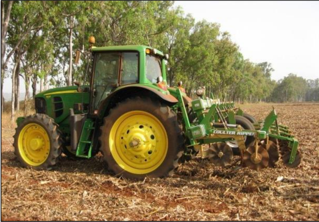
Figure 10. Minimum till machine using coultter ripper for zonal tillage.
