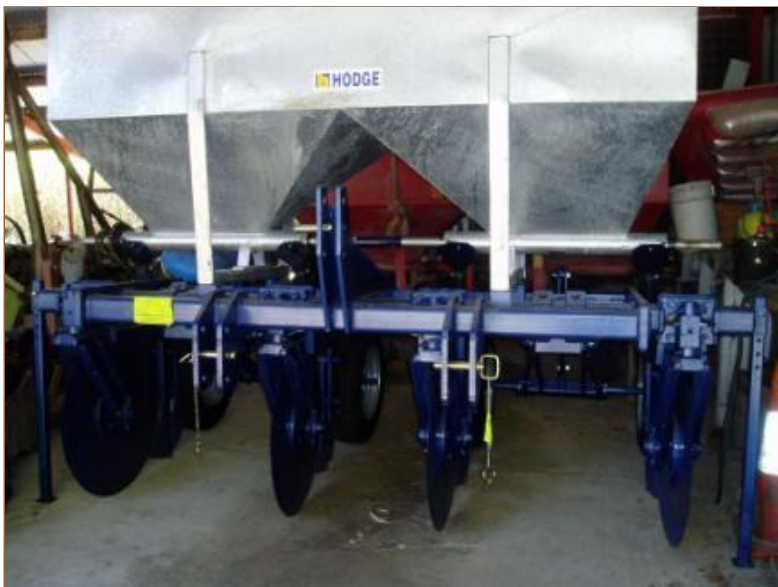
Figure 9. Sub-surface fertiliser applicator places nutrients in the plant root zone.
