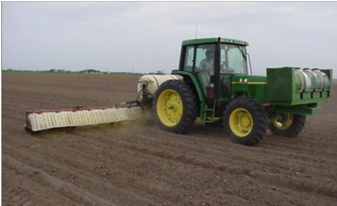
Figure 16. Hooded sprayers reduce spray drift and improve spray efficiency.
