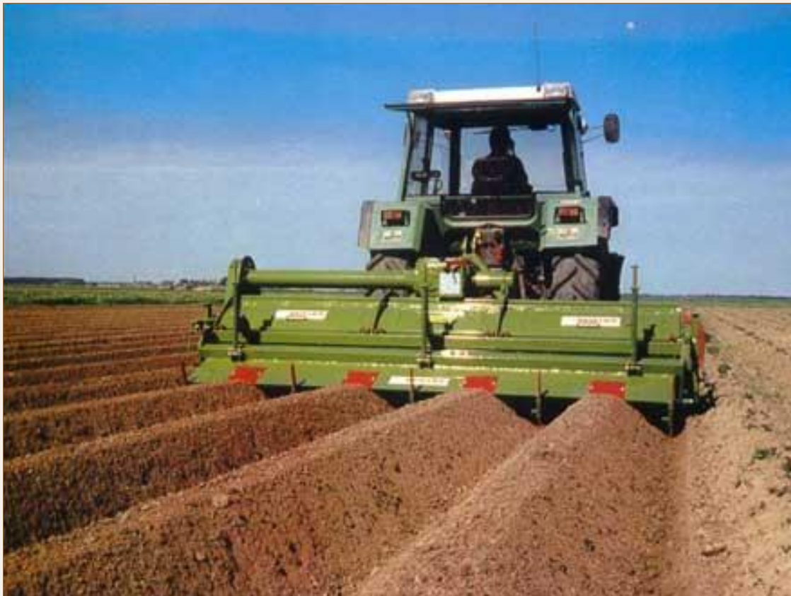
Figure 15. Bed forming is essential for high potato yields to allow good root and tuber formation and drainage.
